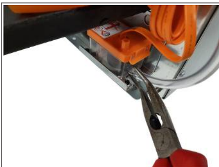
Fig. 42: Loosening the wire clip
