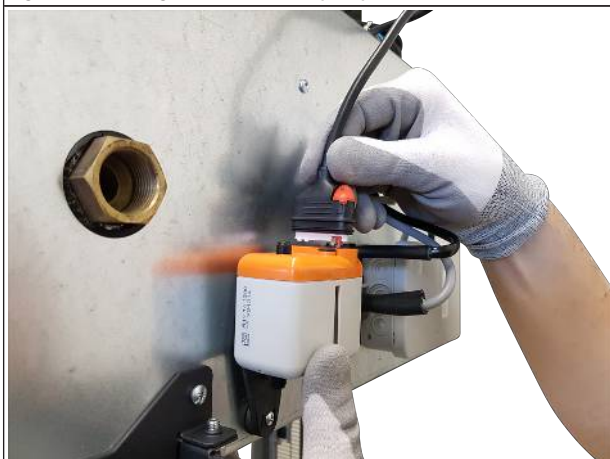
Fig. 26: Connecting to the power supply
