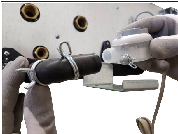
Fig. 23: Fitting the float switch
