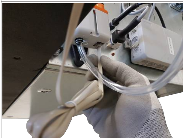
Fig. 29: Inserting the float switch signal cable
