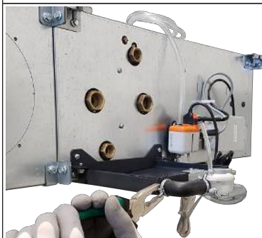
Fig. 58: Loosening the wire retention clamp
