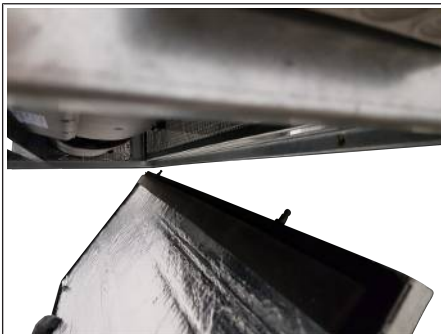
Fig. 53: Inserting the service hatch
